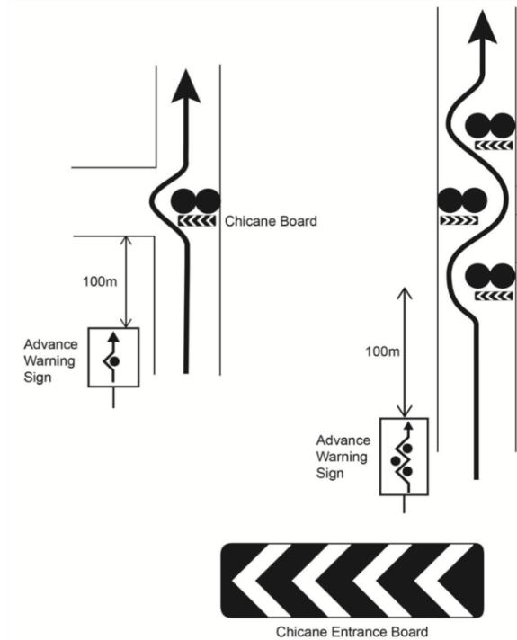
Signage and marks showing the complete position of the chicane elements must be put in place before the beginning of reconnaissance.
